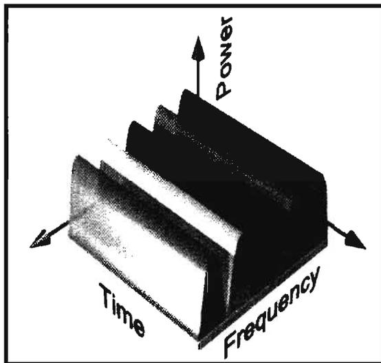
Fig. 1. Time-Frequency Spectra of OFDM
