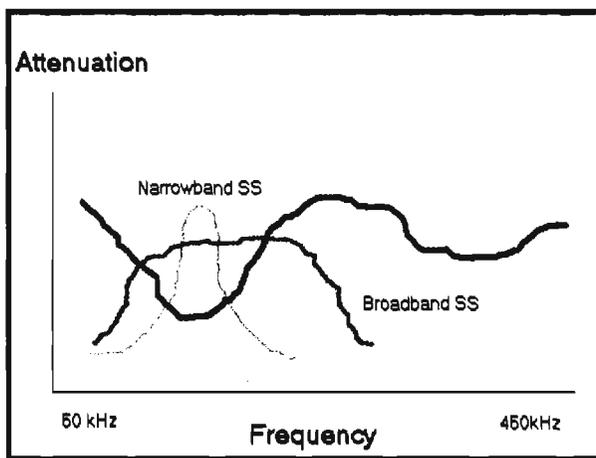
Fig. 4. Powerline Attenuation and Spread Spectrum.
